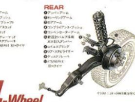
4-Wheel Double Wishbone Suspension
