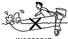
INCORRECT CAUSES BOAT TO "PLOW"
