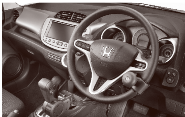
Dタイプ手動運転補助装置(フロア式)フィット装着例 Example of a D-type manual driving assist device (floor-mounted) installed in a Fit
